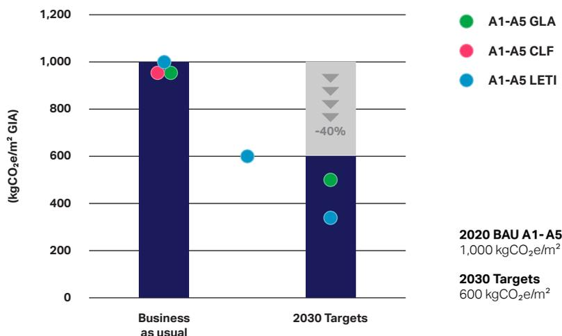
Figure 11 presents current business as usual (BAU) figures in comparison to indicative 2030 targets for upfront embodied carbon and whole life embodied carbon within the industry context.
